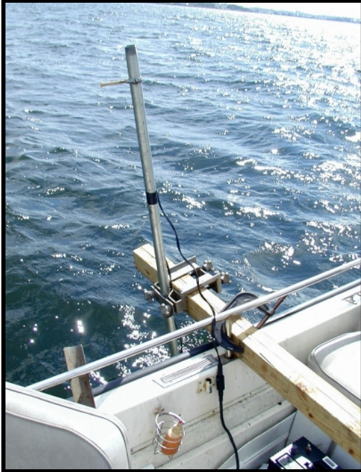
Figure 9-2 Over The Side Transducer Mounting Picture
